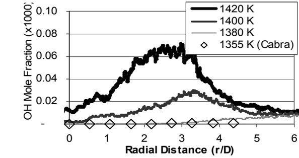
**Figure 3.** Radial profiles at  $x/D = 35$  for coflow temperatures of approximately 1380K, 1400K and 1420K. Point measurements of Cabra (coflow temperature 1355K) are also included.
